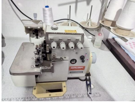
Figure 20 20 maquina overlook industrial
